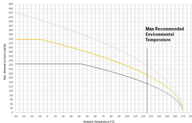
Derating curves may change depending on the final condition of the application (terminals characteristics, wire size etc...).
